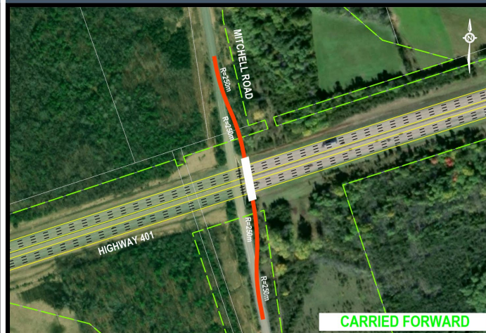
ALTERNATIVE 2 - REALIGNMENT TO THE EAST
