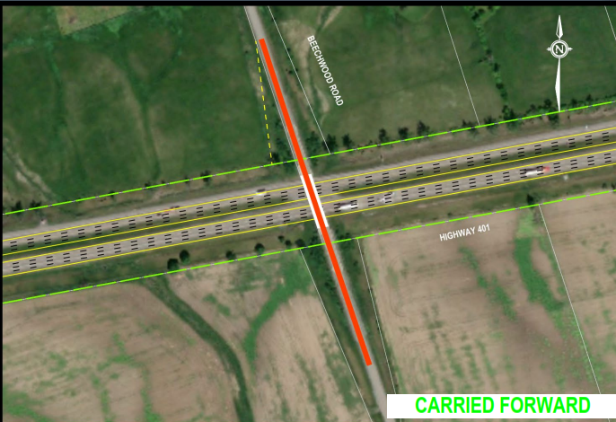
ALTERNATIVE 1 - REPLACE ON EXISTING ALIGNMENT
