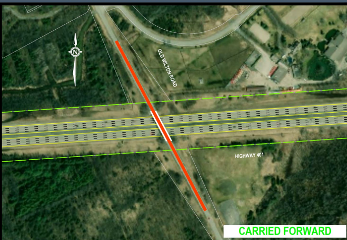
ALTERNATIVE 1 - REPLACE ON EXISTING ALIGNMENT
