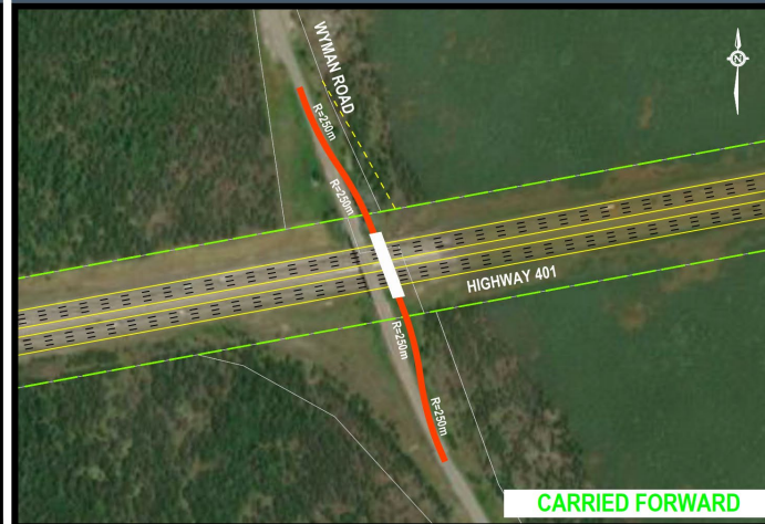
ALTERNATIVE 2 - REALIGNMENT TO THE EAST
