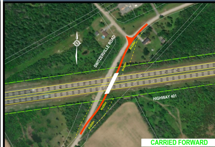
ALTERNATIVE 2 - REALIGNMENT TO THE EAST
