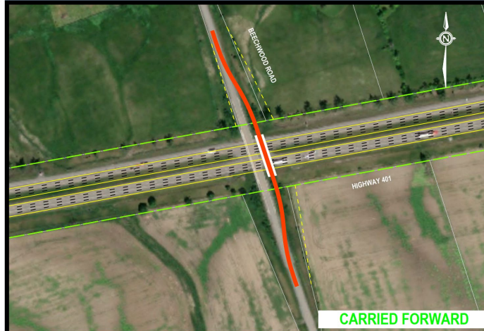
ALTERNATIVE 2 - REALIGNMENT TO THE EAST
