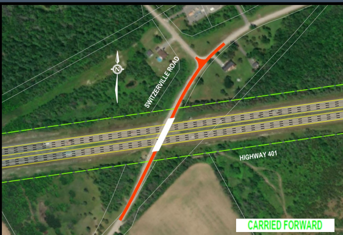
ALTERNATIVE 1 - REPLACE ON EXISTING ALIGNMENT
