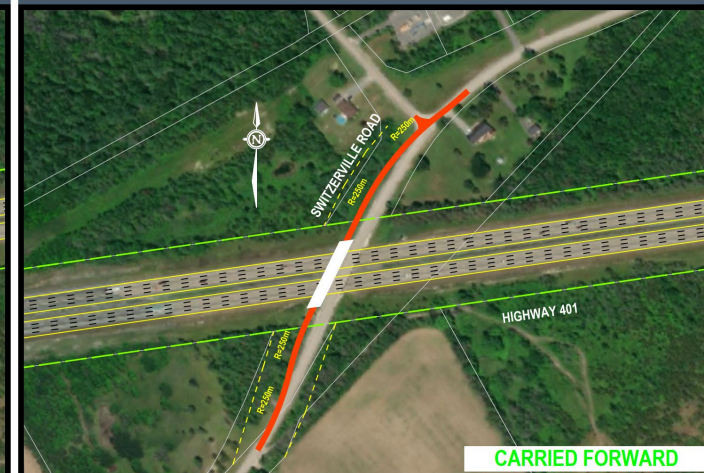
ALTERNATIVE 3 - REALIGNMENT TO THE WEST
