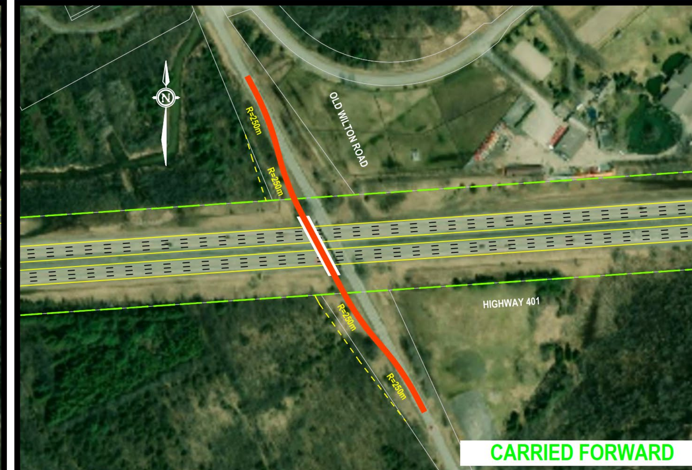
ALTERNATIVE 3 - REALIGNMENT TO THE WEST
