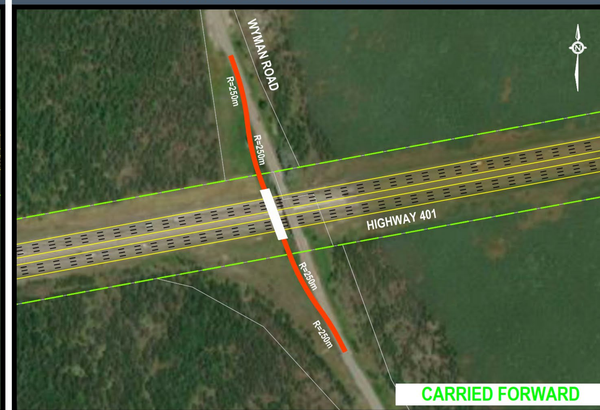
ALTERNATIVE 3 - REALIGNMENT TO THE WEST
