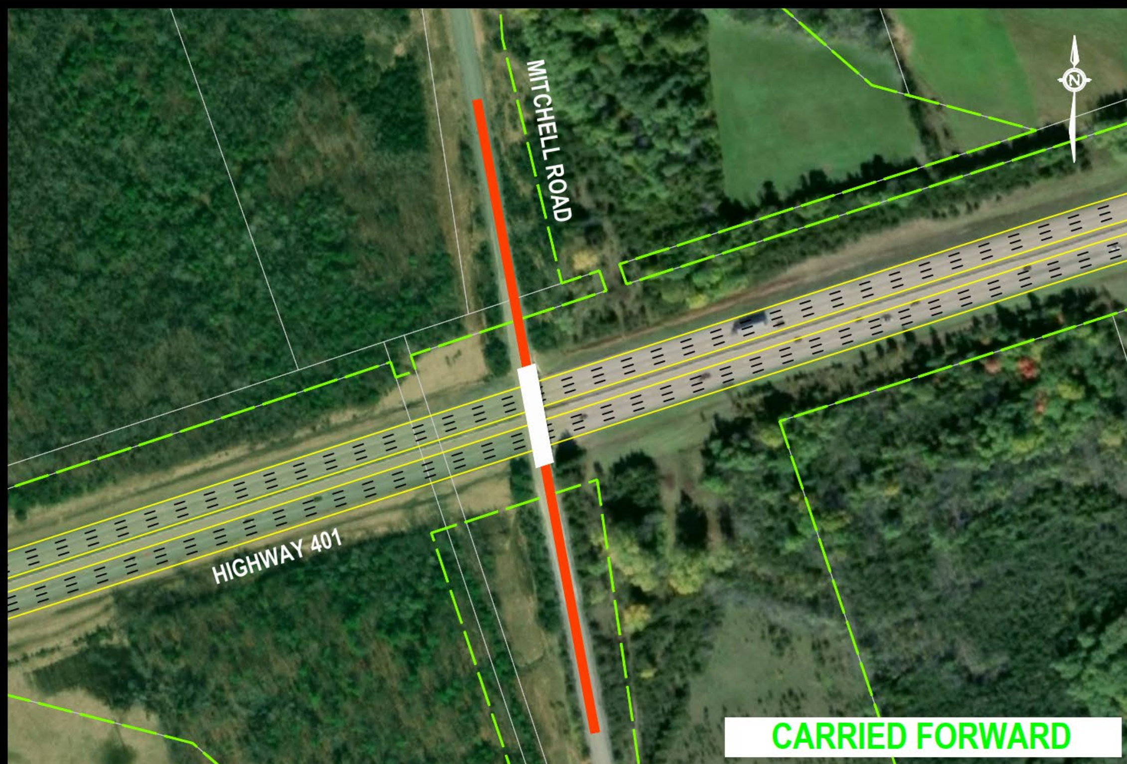
ALTERNATIVE 1 - REPLACE ON EXISTING ALIGNMENT
