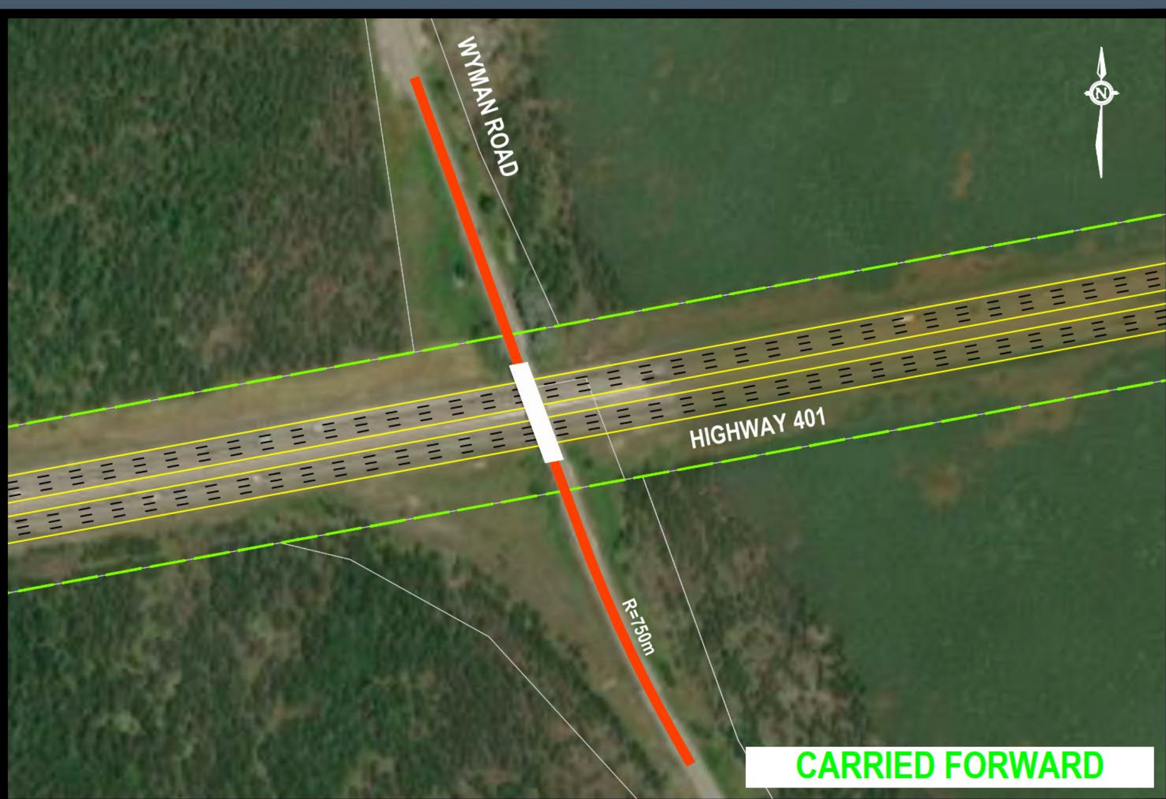
ALTERNATIVE 1 - REPLACE ON EXISTING ALIGNMENT
