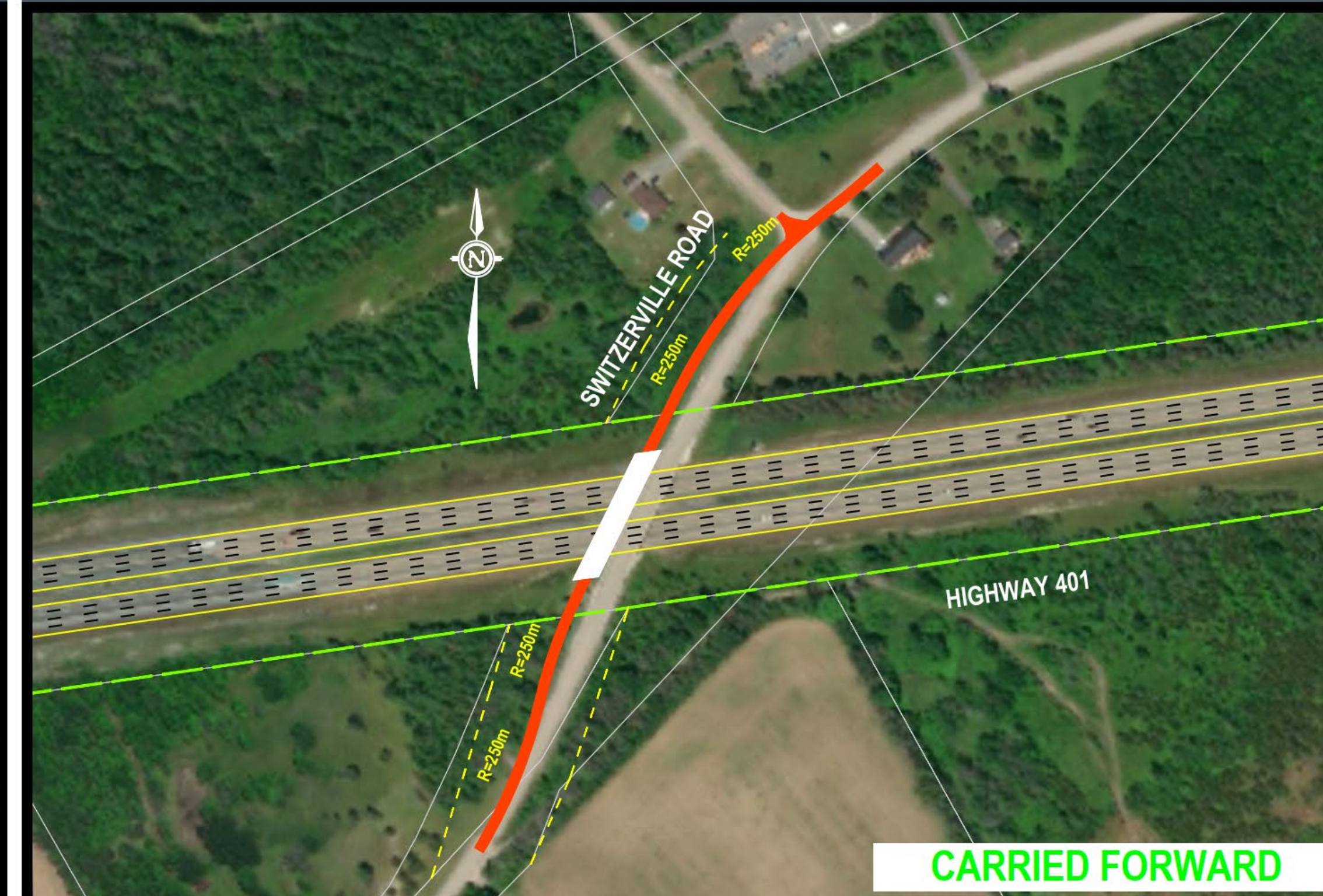
ALTERNATIVE 3 - REALIGNMENT TO THE WEST
